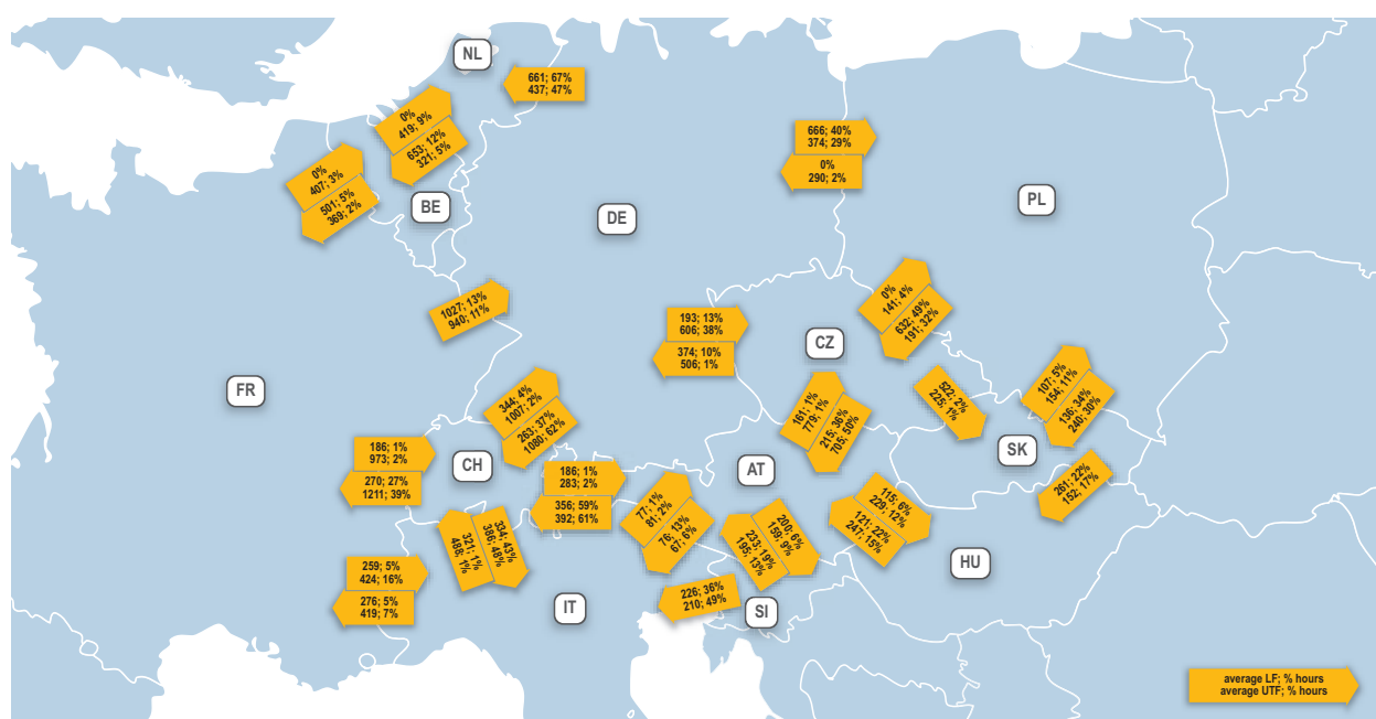
Figure 61: Loop flows and unscheduled transit flows negatively impacting cross-border trade – 2013 (average LFs, UTFs, % hours/year)
