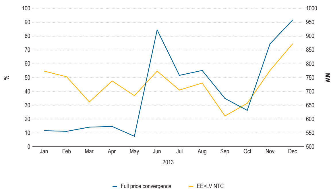
Figure 41: Full price convergence in the Baltic region compared to cross-border capacity (monthly average NTC) from Estonia to Latvia – 2013 (% and MW)
